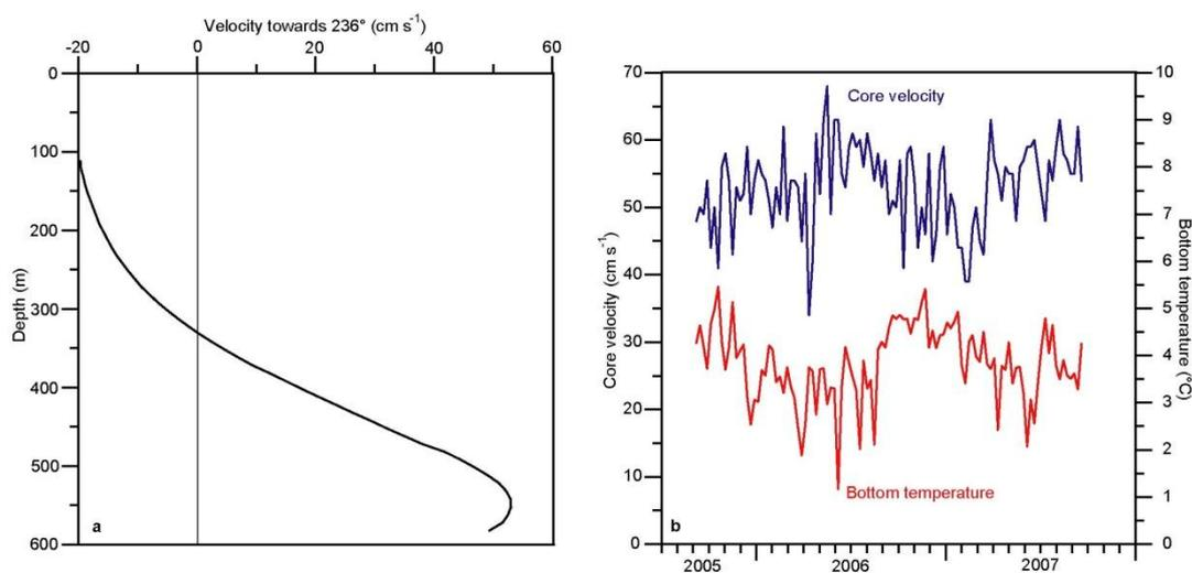
Figure 2. Results from the ADCP at site IFRI (Figure 1) that measured velocity profiles and bottom temperature from September 2005 to October 2007. (a) Vectorially averaged velocity profile towards 236°. (b) Weekly averaged velocity towards 236° for bin 4, approximately 60m above the bottom (blue) and weekly averaged bottom temperature (red).
