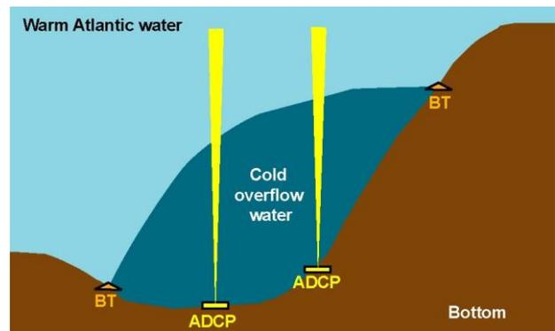
Figure 3. Schematic deployment plan for the field experiment. The two ADCPs will measure vertical and horizontal variation of both overflow and inflow velocity. The two BTs are primarily intended to determine the boundaries of the overflow plume.
