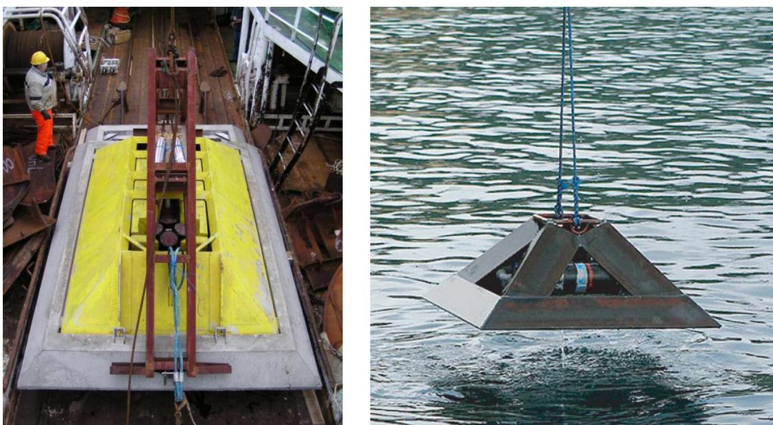
Figure 4. Left panel: An ADCP in a trawl-protective frame (yellow) onboard R/V Magnus Heinason, ready for deployment. Right panel: A bottom temperature measuring unit (BT) including temperature sensor, acoustic modem, and batteries in a trawl-protective frame.
