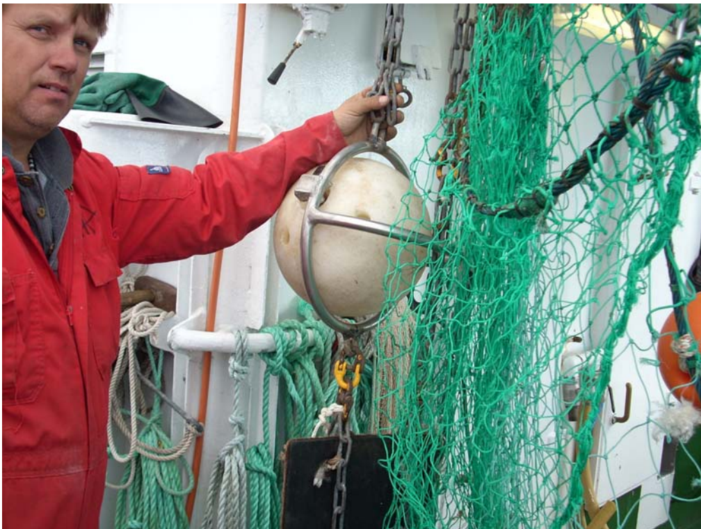
Figure 5. 11" plastic bobbins mounted in the same frame as the steel bobbins showed in Figure 4.
