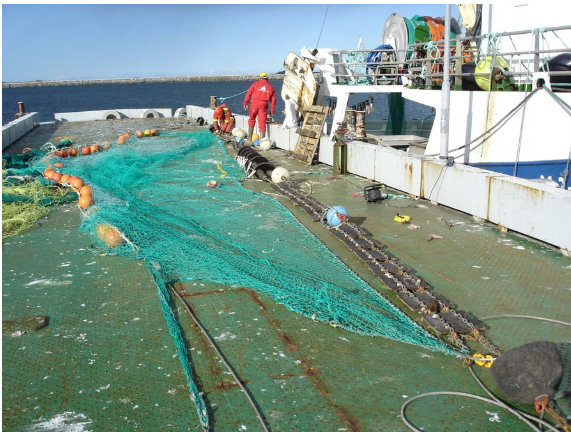
Figure 2. The ground gear used for the experiments
