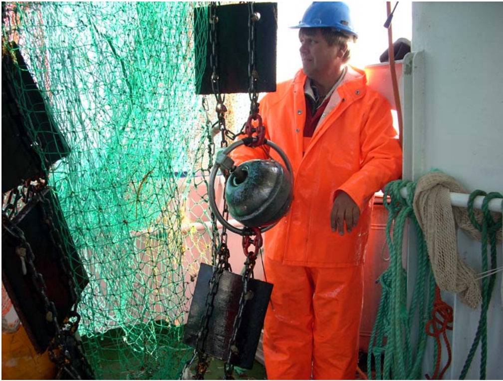
Figure 4. 9" steel bobbins mounted in a circular steel frame with a shaft as diameter.
